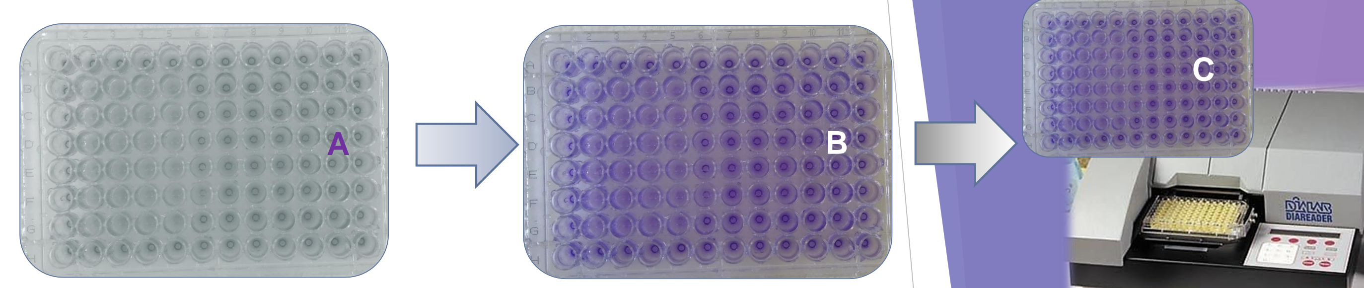
Fig. 1 Schematic O'Toole's modified method on biofilms in a microtiter plate. Biofilm formation in 96 well microtiter plate during the incubation and washing (A), treatment with crystal violet and washing (B), suspending of the dyed biofilm in acetic acid and its transfer to a new microtiter plate, absorbance measurement at 544 nm with DIALAB EL800 microplate reader (C).
